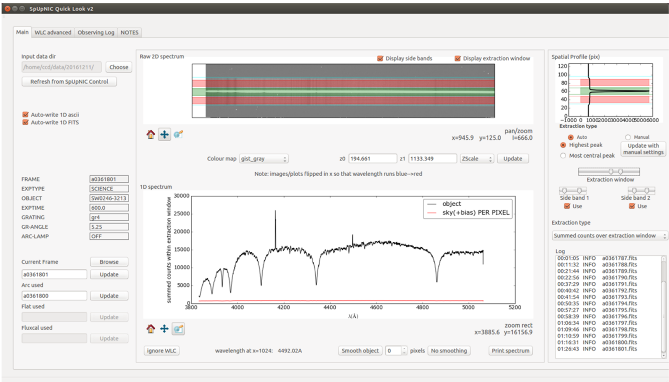
Fig. 5 Screenshot of the SpUpNIC quick-look GUI, displaying an object spectrum that has been extracted, sky-subtracted and approximately wavelength calibrated.
